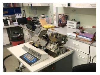
We are continuing to work through the PCs and PS2s we received recently. Several machines are now in good working order. Where we have been unsuccessful is generally down to power supply issues. Unless it's obvious, like an exploded capacitor, it is difficult to fault find without wiring diagrams.
